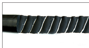
Pic 3: Sample with an excellent adhesion
