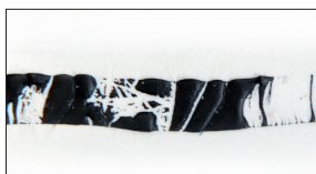
Pic 4: Good adhesion with some cohesive failures in the substrate
