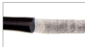
Pic 5: Bad adhesion. Nothing or a thin film remaining on the substrate
